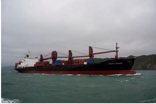
Conventional ship, onboard cranes
